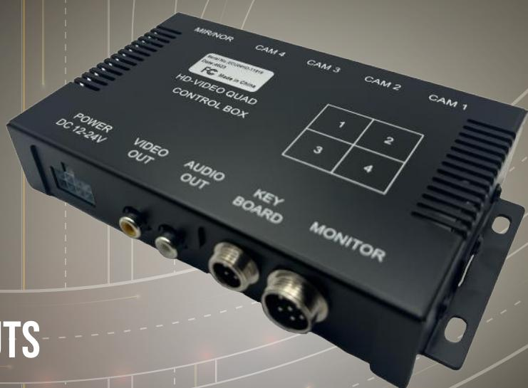
Introducing the ECU04HD a revolutionary HD Video Quad Control Box tailored for commercial trucking. It seamlessly integrates up to four SD/HD cameras into one output channel, providing crisp HD quality video at AHD 720p 30fps. Its compact design, measuring just 6.5" x 4.1" x 1", simplifies installation, while the inclusion of both BNC and 4-pin DIN parallel outputs ensures versatility.
